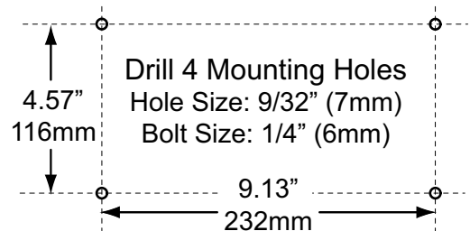
Figure 2: Drill Pattern and Hardware
