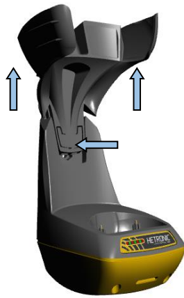
Figure 17. Pulling the gripper upwards whilst keeping the clip pressed
